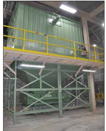
Geelan pellet cooler, one of the largest models available.
