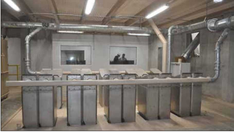
CPM Beta Raven 20-bin microingredient system, with control room visible behind it.
